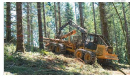
especially in the spring and fall. Loggers can overcome these obstacles with Cat forwarders, designed to transport large payloads long distances over difficult terrain. Cat equipment also gives customers the ability to construct access and hauling roads into forestry work areas.
